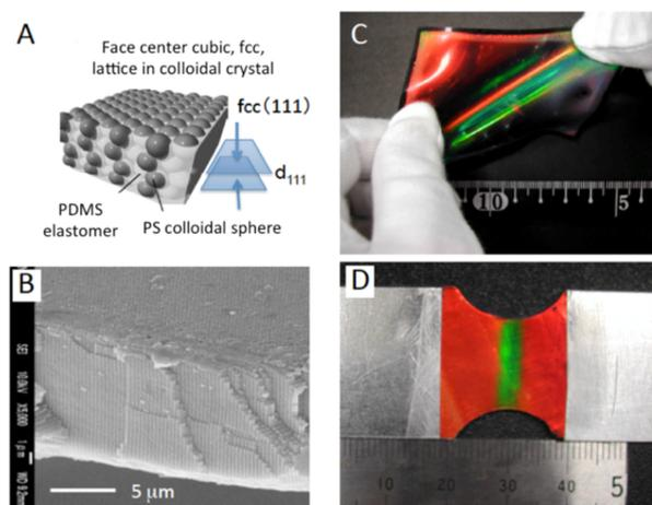
**Figure 1.** Soft opal photonic crystal films. (A) PS colloidal crystal of fcc (111) planes embedded in PDMS elastomer. (B) SEM image of the soft opal film. (C) Color changing by stretching a rubber sheet. (D) Strain image of deformed aluminium plate.
