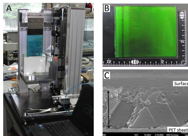
**Figure 2.** Crystal growth of opal photonic crystal film. (A) Vertical coating equipment based on oil covering method. (B) Optical image of opal photonic crystal film coated on a PET sheet. (C) Cross sectional SEM image of the opal film made of closely packed 200nm-PS colloids.
