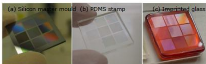
Fig. 1. Arrays of pillars, lines and holes were developed using a conventional photolithographic processes into Si wafer substrate. This was then used as (a) a master mould for creating (b) the PDMS replica (soft stamp). Part (c) shows the individual arrays imprinted into chalcogenide As-S bulk glass.
