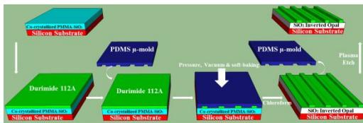
**Fig. 2.** Waveguide fabrication process.
