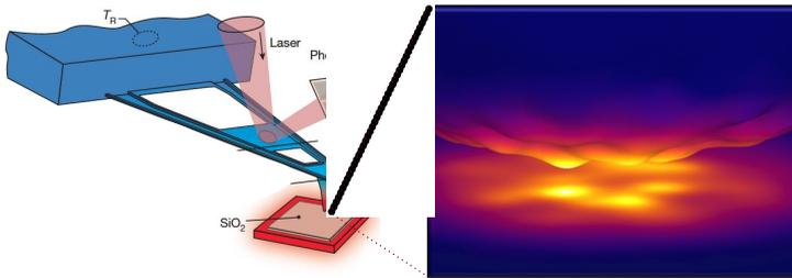
**Fig. 1.** Radiative thermal radiation between an AFM tip and a surface both made of  $\text{SiO}_2$  and separated by a few nanometers.
