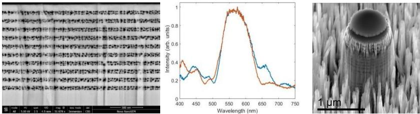
**Fig. 1.** Left: SEM micrograph of a porous GaN distributed Bragg reflector, fabricated on the non-polar a-plane. Centre: corresponding reflectivity trace, showing a peak reflectivity of 98%. Right: Porous GaN incorporated into an etched micropillar cavity, with roughening of the etched surface due to the porous structure.
