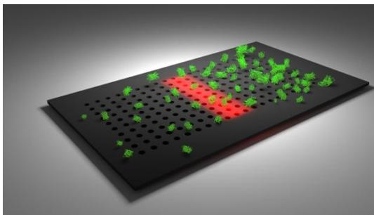
**Fig. 1.** Artist's impression of a photonic crystal biosensor that affords a simple camera readout, as the resonance is localised in a certain part of the photonic crystal depending on the local refractive index; as the index changes due to, e.g. the attachment of biomolecules, the resonance moves to a different position on the chip.
