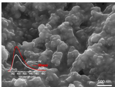
**Fig. 1.** Morphology of ZnO-PDMS nanohybrids is shown.
