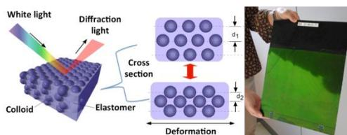
**Fig. 1.** Colloidal photonic crystal film with tunable structural color. Left: Tuning periodic structure by mechanical deformation. Right: High quality colloidal photonic crystal films coated over 1000cm<sup>2</sup> on a black color PET sheet.
