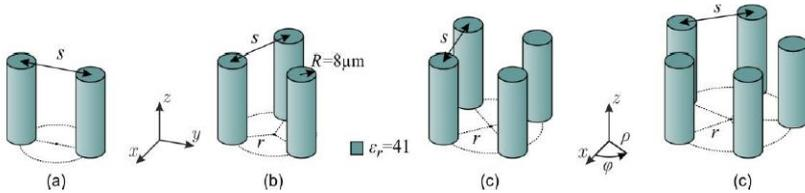
**Fig. 1.**  $N$  identical polaritonic rods of radius  $R=8\mu\text{m}$  are located at the vertices of regular polygons.
