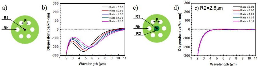
**Fig. 1.** (a) Conventional structure of chalcogenide HMOFs and (b) the calculated chromatic dispersion with  $\pm 10\%$  fiber structure fluctuation. (c) New structure of chalcogenide HMOFs and (d) the calculated chromatic dispersion with  $\pm 10\%$  fiber structure fluctuation. The core diameter, buffer diameter and air-hole diameter are R1, R2 and Rh, respectively. The distance between the two air holes is depicted by P.
