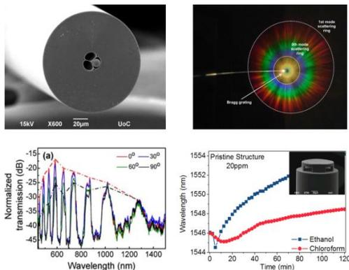
**Fig. 1.** (top left) microspherical resonator encapsulated inside a microstructured optical fibre; (top right) out-scattering light from a relief Bragg gratings reflector inscribed inside a photonic crystal fibre; (bottom left) transmission bands from an all-solid photonic band gap fibre, exhibiting plasmonic properties; (bottom right) sensing behavior for ethanol and chloroform of a fibre endface Fabry-Perot sensor fabricated using multi-photon polymerisation.
