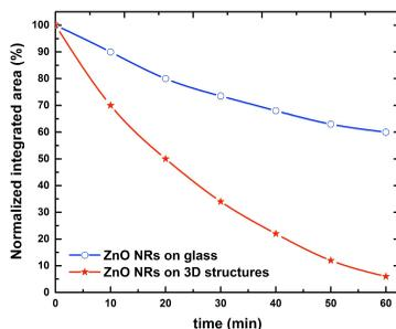
**Fig. 2.** Normalized absorption of aqueous solution of methylene blue at  $\lambda_{\max}=665$  nm under UV light irradiation for ZnO nanorods grown on glass substrates (blue circles), and ZnO nanorods on 3D structures (red stars), respectively.
