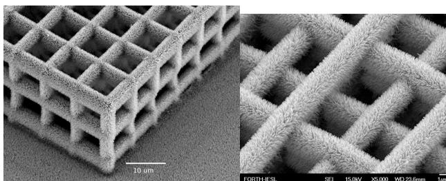
**Fig. 1.** 3D structures covered with ordered ZnO nanorods.
