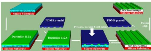
**Fig. 2.** Waveguide fabrication process.
